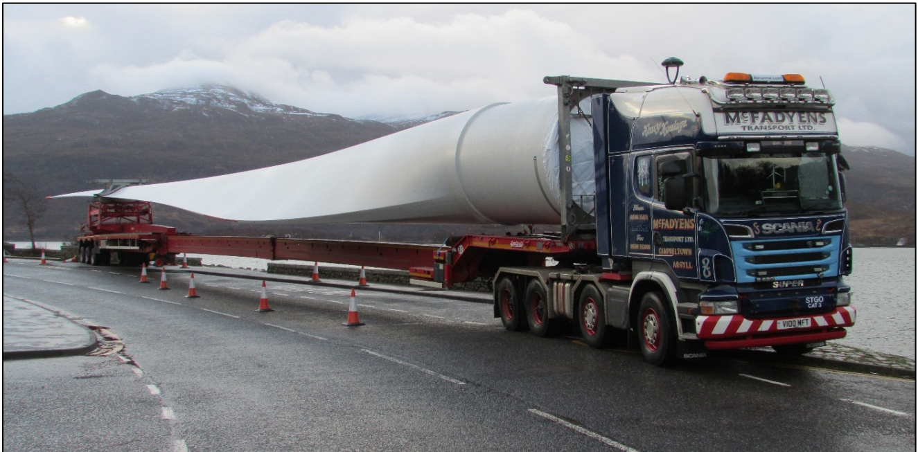
Figure 2-2: Superwing Carrier Trailer
